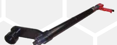
860 mm Nose extension, cranked torque reaction & 2,000 N-m tool for long reach Wellhead connectors
