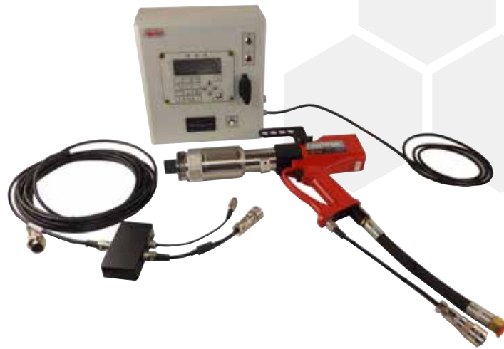
Torque & angle bolting kit, 2,000 N-m. Tighten to torque & then to specified angle to put bolts into yield
