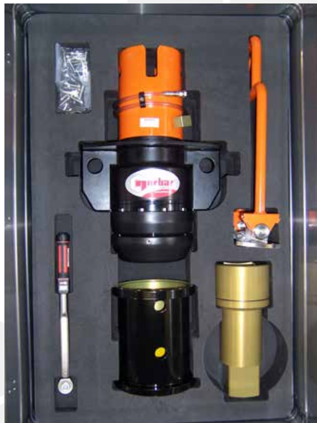
API 17D 4 - 6 / 4 - 7 / 4 - 7 short interchangeable kit 34,000 N-m
