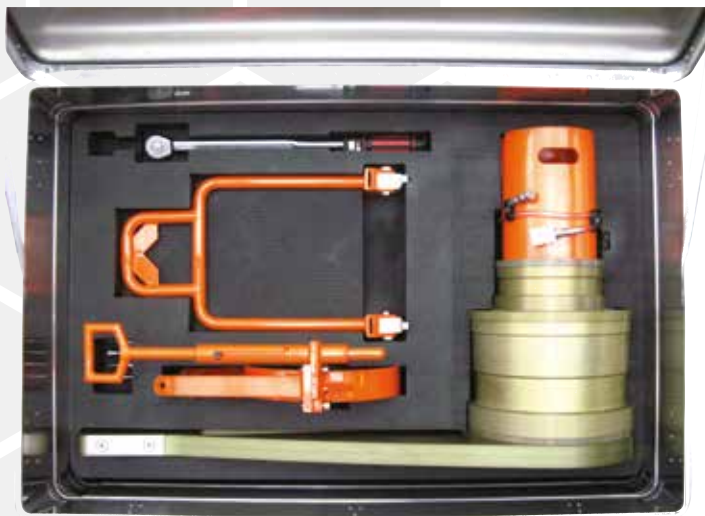
63,000 N·m wet pipe clamp tool
