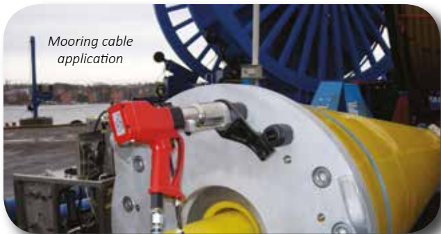
PneuTorque® fitted with torque transducer and angle encoder, shown with torque and angle or turns measuring instrument.
