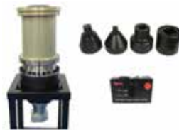
Transducer calibration rigs 100,000 N-m rig example
